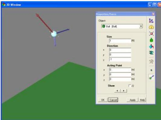
Double-clicking on the Force's blue arrow brings up the Properties dialog. From this dialog, you can set the force's parameters. Set the two constant forces with the help of this panel. The first vector should be a force of 1N, and its direction  $x = 0$ ,  $y = 0$ ,  $z = -1$ , pointing downwards. The second vector's force should be 2N, and its direction  $x=1$ ,  $y=0$ ,  $z=0$ , (horizontal).
