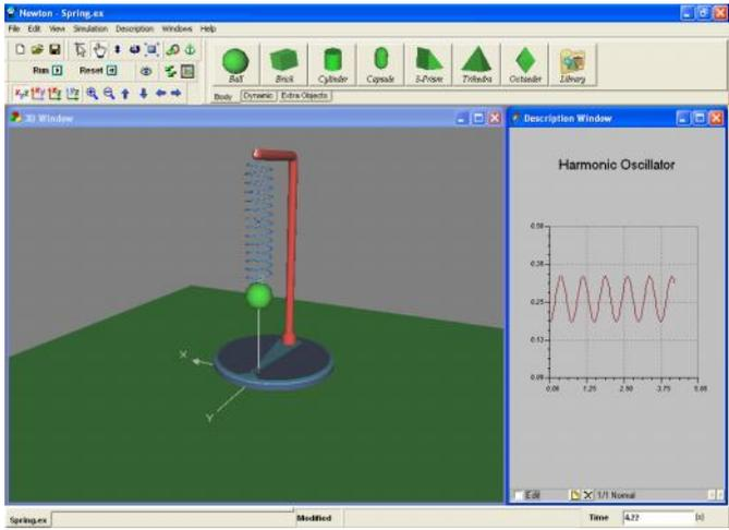
The unstrained length of the spring can be set while viewing the 3D window. Lift the ball to the desired unstrained position, click on the spring with the right mouse button, and select the unstrained length command from the context menu. This results in the actual size of the spring also being the unstrained size.
