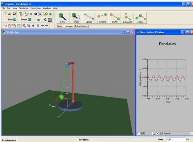
Go to the Properties window where the hinge's parameters are set. You can draw any of these parameters on a diagram, and they all can be reached from the Diagram dialog. In the diagram window above we have presented a curve showing the angle of swing of the pendulum.
