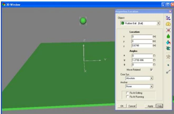
Click on the
