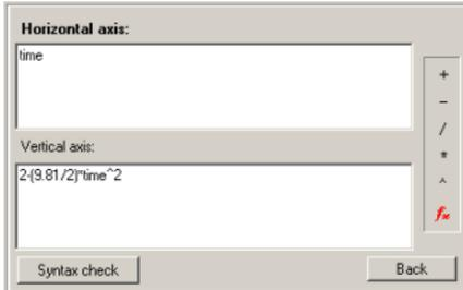
The word 'time' defines the horizontal axis variable to be the simulation time. The vertical axis is assigned the expression  $2-(9.81/2)*time^2$ , written as the equation  $z=z_0-\frac{1}{2}\cdot g\cdot t^2$  in Newton. The term  $z_0=2$  is the initial position of the ball.
