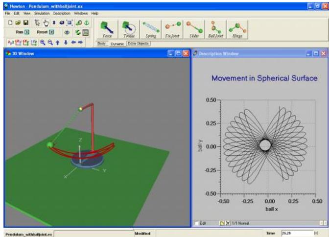
From the Properties Window, you can set all the balljoint parameters to exact values. Any of these parameters can be plotted as curves on the diagram. The picture above graphs the ball's position in the x–y plane.
