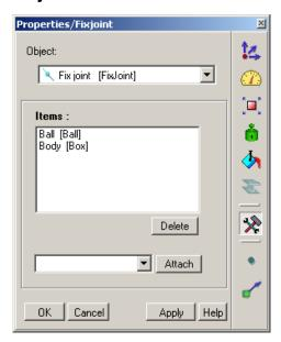
The Items list displays the linked objects. Additional objects can be linked to the fixjoint by selecting the object from the combo box below the list, and clicking on the Attach button.
