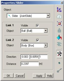
The slider object links two bodies. The **object** combo box shows these two bodies, and permits you to select another object from the list. Select 'none' to break the original link to the object.
